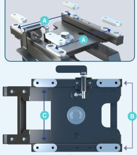
Top view swivel unit of the leg with spacers
